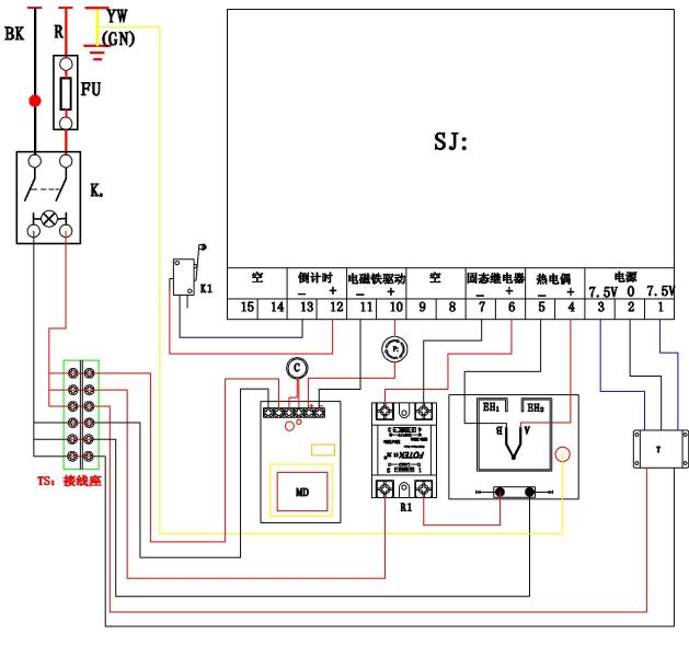
K<sub>0</sub>: Power Switch SJ: Digital Controller C:Magnet K1:Limit Switch MD:Magnet Driver
